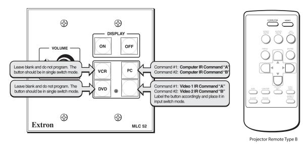
Programming an MLC 52 VC model with a projector remote control type B
